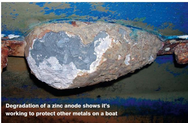
Degradation of a zinc anode shows it's working to protect other metals on a boat
